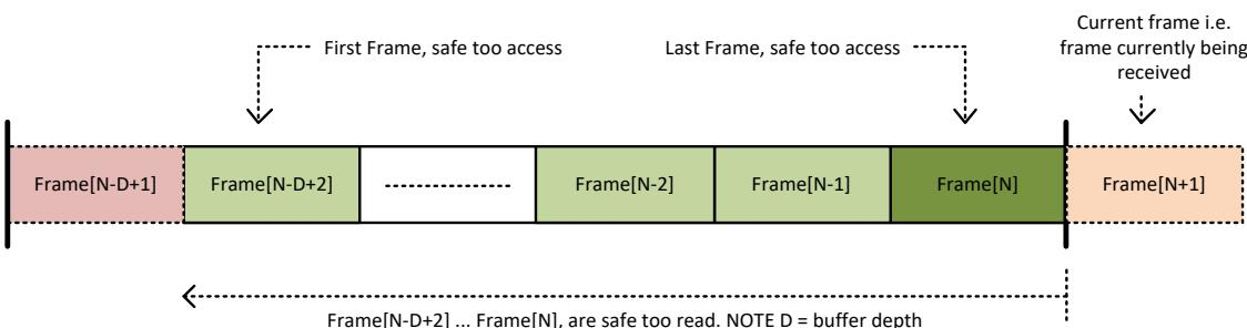
In case of output mode *CurFrame* indicates the frame that is currently being transmitted (i.e. it is safe to write to the frames:  $CurFrame + 1 \leq Frame \leq CurFrame + (D - 1)$ ).
