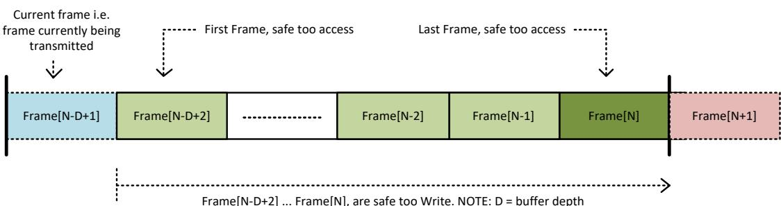
NOTE: use `DtFrameBuffer::GetBufInfo` to determine the depth (#columns) of the frame-buffer.
