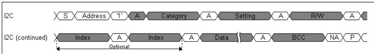
Figure 7 below shows the sequence to send a command over I<sup>2</sup>C to the DTM-3200. If the command is a read-command, the data may be omitted. If the category does not require an index, the index must be omitted.
