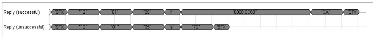
Figure 11: Reply after a device type read-command
