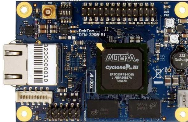
Figure 1. The PCB of the DTM-3200
