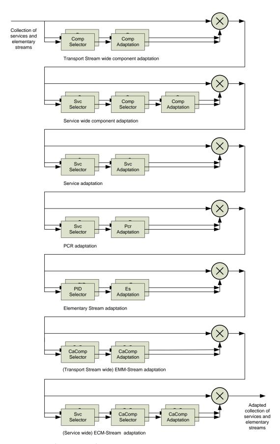
Figure 13. Illustration of adaptation of the output stream.
