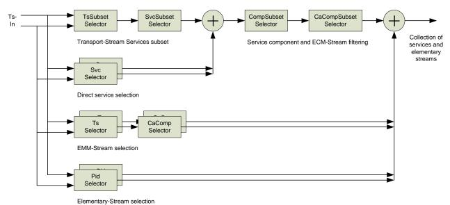
Figure 5. Illustration of the Transport-Stream wide composition.
