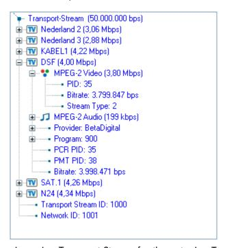
To select a service from an incoming Transport Stream for the outgoing Transport Stream, place the mouse cursor over the icon of the desired service and hold the left-mouse button down while dragging the service to the output.
