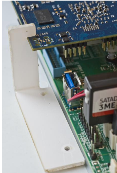
Figure 4. Custom-made support part.
