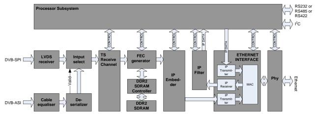
Figure 5: Functional block diagram of the DTM-3200 when configured as ASI-to-IP converter
