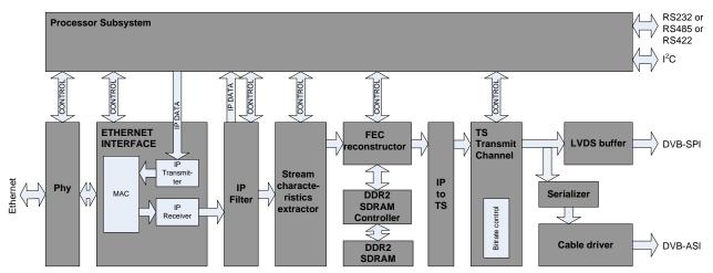
Figure 4: Functional block diagram of the DTM-3200 when configured as IP-to-ASI converter
