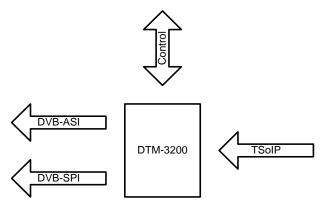
Figure 2. The DTM-3200 configured as IP-to-ASI converter
