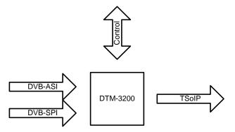
Figure 3. The DTM-3200 configured as ASI-to-IP converter
