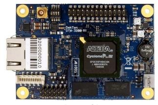
Figure 1. The PCB of the DTM-3200
