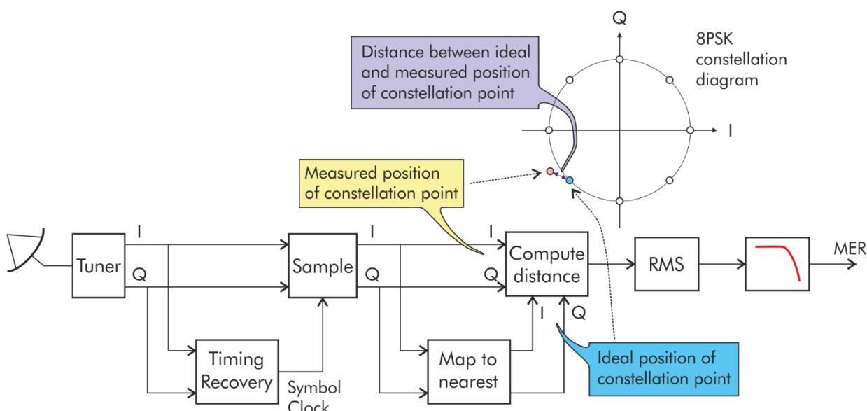
**Note:** If the signal power is low or there is a lot of noise (low value of SNR/MER), the nearest constellation point may not always be the correct one. The demodulator will correct the error, but it will not reconstruct the originally intended symbol. What this means is that at very low SNR/MER, the MER estimate of the demodulator will be a bit too high. The actual MER is lower (=worse) than the MER estimate.
