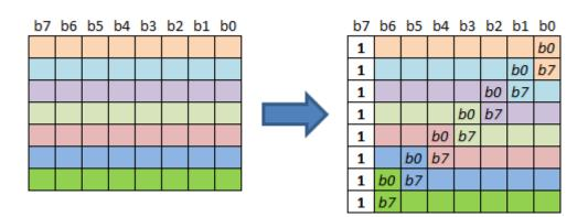
Figure 6. ASCII encoding for firmware update data
