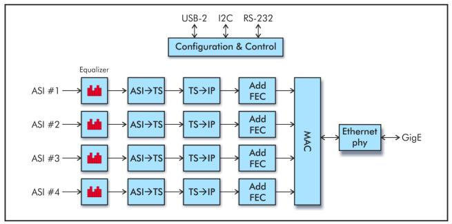
Figure 3: Functional block diagram of the DTM-3224
