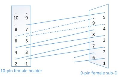
An I<sup>2</sup>C controller can be connected to SDA and SCL on pin 9 and 10, with signal ground on pin 7.
