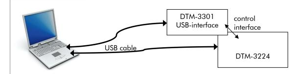
Connect the DTM-3224 to the power-supply using the power connector (see §3.2.7). The DTM-3224 will boot which will take a few seconds. During this time the LEDs on the DTM-3224 are green. Wait until the DTM-3224 input LED's start flashing green.
