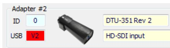
In USB-2 mode, the DTU-351 is visible in **DtInfo** and VPD data can be read, but the DTU-351 cannot transfer HD-SDI or other data at all.
