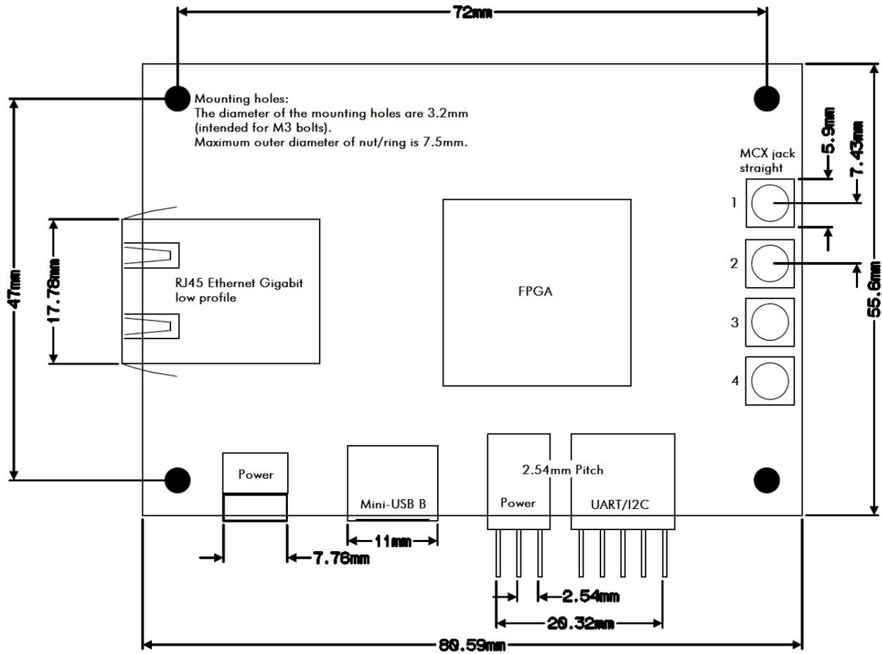
**Warning:** While mounting the DTM-3224, care should be taken not to damage components that are close to the mounting holes, both on the top and bottom side of the board.
