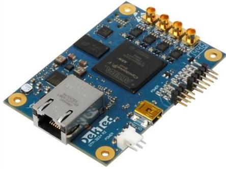
A blue printed circuit board (PCB) with various electronic components. It features a large black integrated circuit (IC) in the center, several gold-plated SMA connectors along the top edge, a USB Type-A port on the left, and a white multi-pin connector at the bottom. The board is populated with various surface-mount components like capacitors and resistors. | DTM-3224 without accessories |
