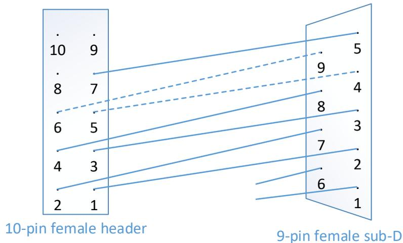
An I<sup>2</sup>C controller can be connected to SDA and SCL on pin 9 and 10, with signal ground on pin 7.
