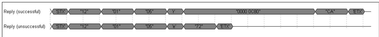
Figure 9: Reply after a device type read-command
