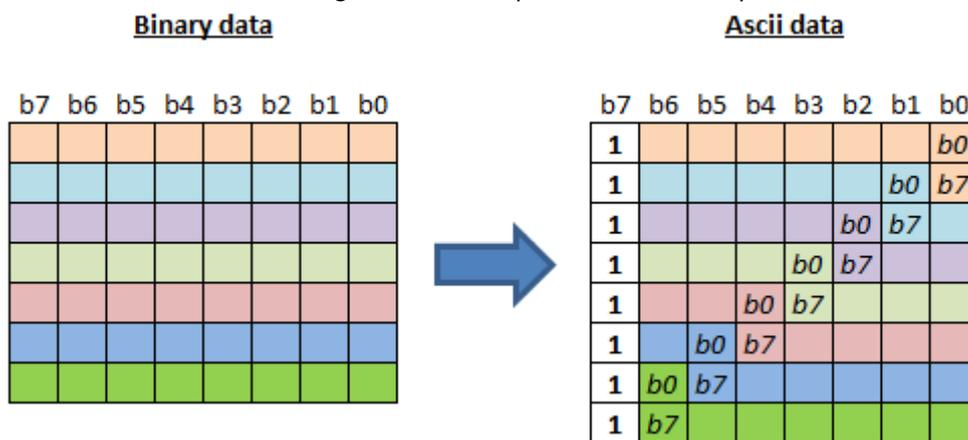
Figure 6. ASCII encoding for firmware update data
