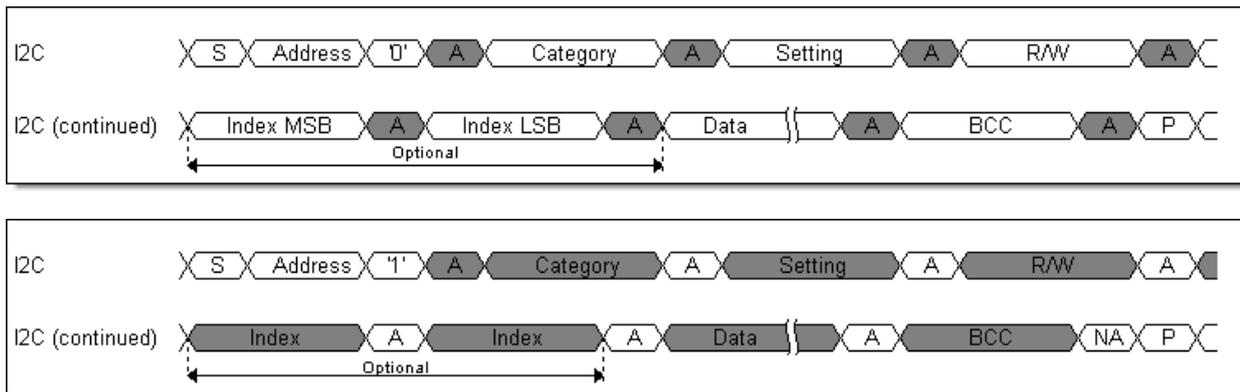
Figure 5. Command (upper sequence) and response (lower) sequence for I<sup>2</sup>C
