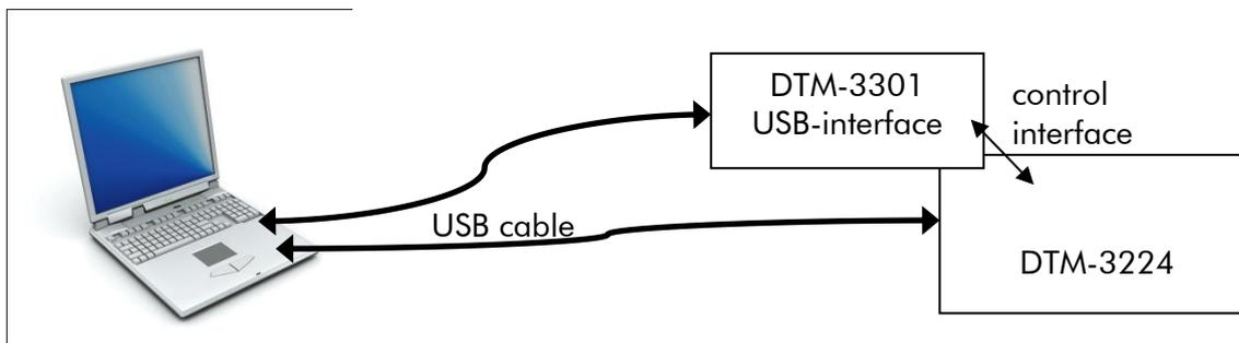
Connect the DTM-3224 to the power-supply using the power connector (see §3.2.7). The DTM-3224 will boot which will take a few seconds. During this time the LEDs on the DTM-3224 are green. Wait until the DTM-3224 input LED's start flashing green.
